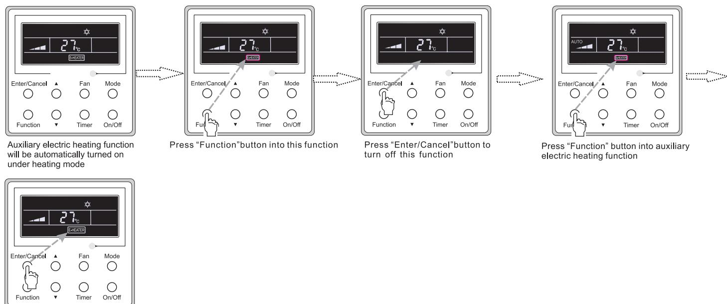
Fig.12 E-heater Setting
