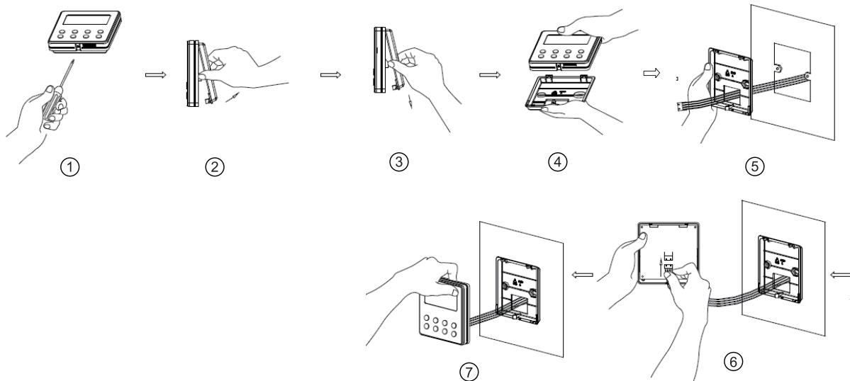
Fig.15 shows the installation steps of the wired remote controller, but there are some issues that need your attention.
